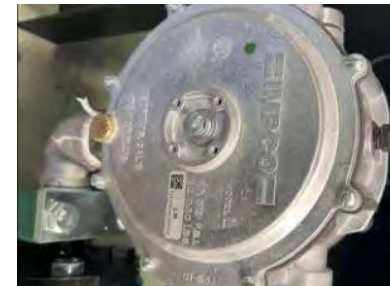
IMPCO Regulator Model L | W.P.312PSI
